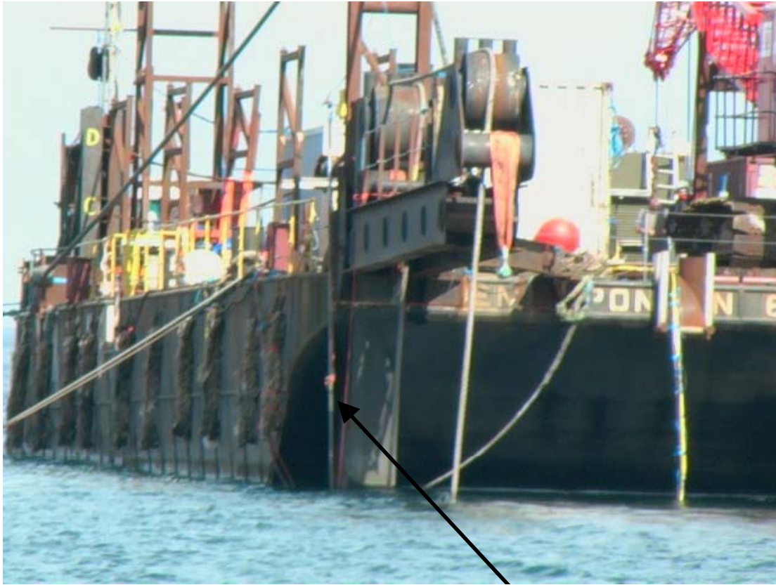
Plate 4. Location of remote POD rig on barge. The scaffold pipe housing the hydrophone cable is indicated just to the left of centre picture. Stingray is deployed on the seabed 35 m below the stern of the barge in view.
