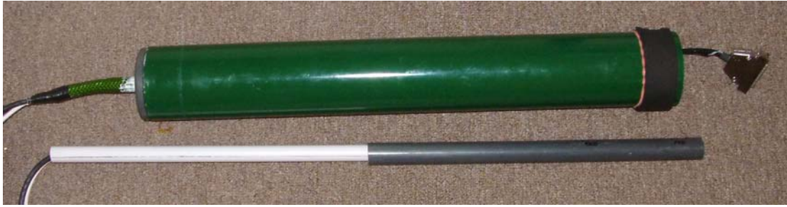
Plate 1. Barge POD, with data cable and lead to remote acoustic sensor (in foreground)
