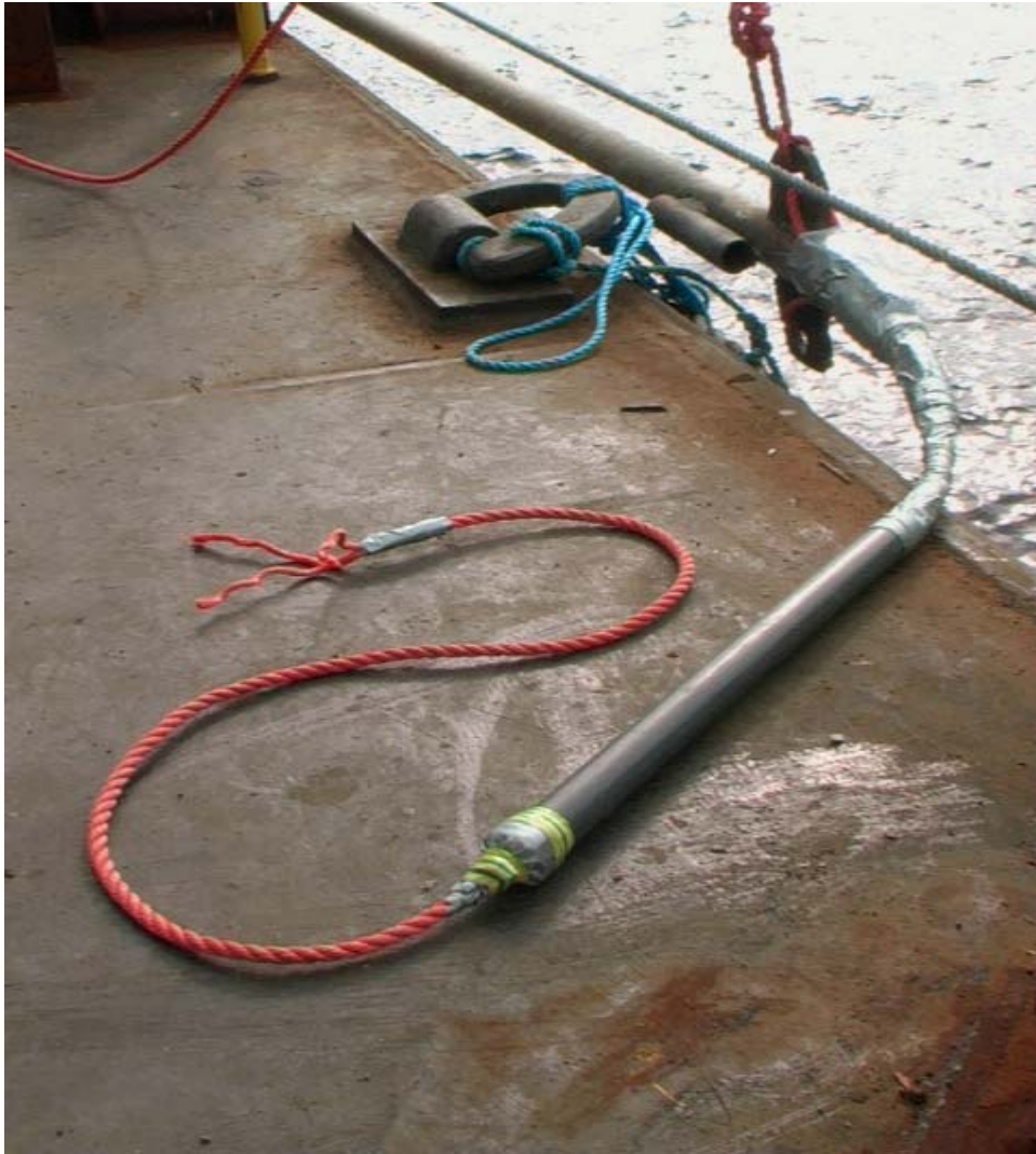
Plate 5. Trailing hydrophone on the barge deck.
