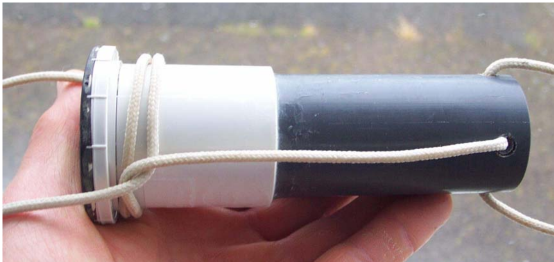
Plate 2. A self-contained experimental porpoise alerting device (PAD)
