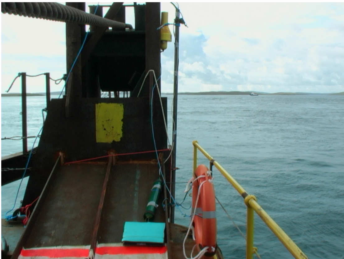
Plate 3. Remote POD unit housing PAD electronics with laptop set up on the deck of Stingray barge. The 6 m length of vertical scaffold pipe houses the hydrophone and PAD cable with the hydrophone secured 30 cm below the hull of the barge.
